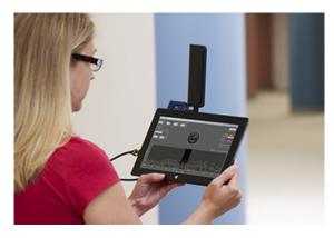
In general, portable analysis should be one of the last steps taken when tackling Wi-Fi problems. Step one should be verifying the settings configured on the user's device(s). Step two should be ensuring that the wireless LAN infrastructure has been set up according to sound RF principles. Once those two steps have been taken, step three should be to use a portable wireless analyzer.
